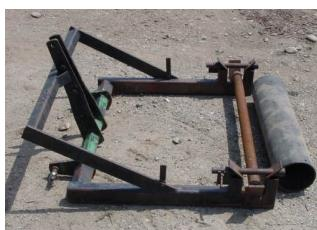
The simplest type of big roll sod layer is the 3-point hitch, which is shown in the 3rd Photo to the Left. This type of layer attaches to the three-point hitch of a tractor. It will NOT hook to a skid loader. It is a very inexpensive installer but requires more operator skill. Also, the tractor tire will make impressions on some soil types. *(Continued on back side,)*
